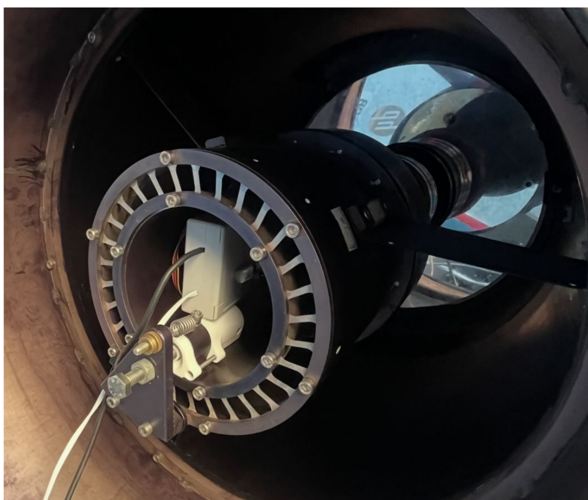
Figure 3: Interim focusing mechanism for ROTSE-IIIc, replacing the original micrometer with a linear actuator housed in a custom 3D-printed mount.
